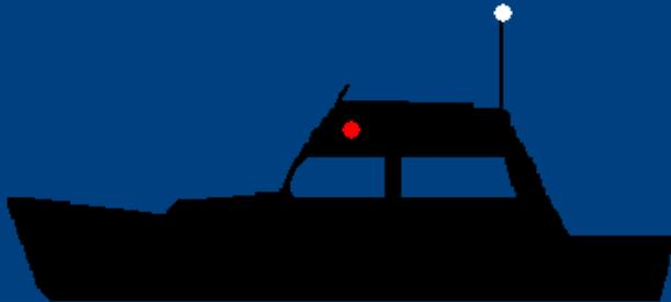
Viewing the vessel from its port side.
